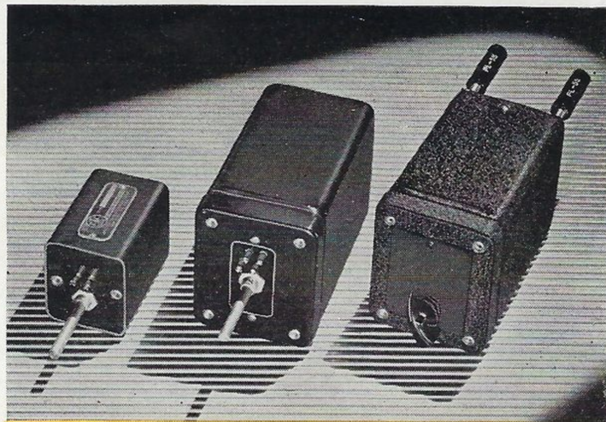
Equalizers with built in control are frequently advantageous. Left to right: Special equalizer with built in tap switch—Special equalizer with built in T pad for control — selectable band pass—band eliminator filter made for U. S. War Dept.
